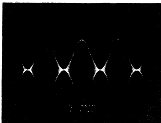
FIGURE 3 -- AMPLITUDE-MODULATION OUTPUT WAVEFORM
